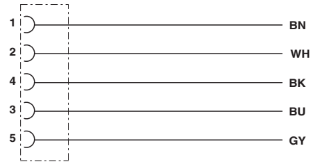
Contact assignment of the M12 socket
